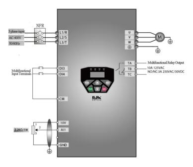
Figure 5-3 Wiring Diagram
