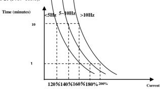
Fig 6-21 Motor overload protection value
