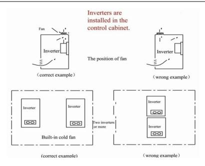
Fig 1-2 Installed in the cabinet
