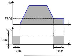
Figure 5-18 DC braking
