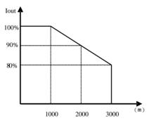
Fig 1-1 Derating drive's output current with altitude
