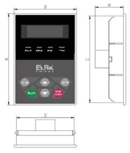
Fig.3-4 Operation Panel Structure
