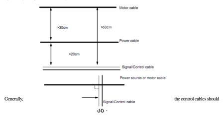
be shielded cables and the shielding metal net must be connected to the metal enclosure of the drive by cable clamps.
