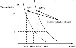
Fig 6-20 Motor overload coefficient
