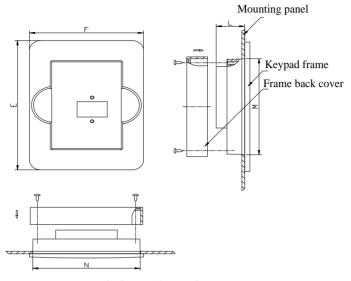
Fig.3-6Panel mounting structure
