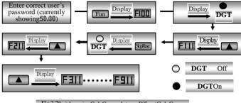
Fig 3-7Switch over in a Code Group or between Different Code-Groups
