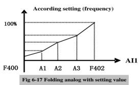
F400 and F402 are lower/upper limit of analog AI1 input. When F460=1, F462=2.00V, F463=1.4, F111=50, F203=1, F207=0, then A1 point corresponding frequency is (F463-1) \*F111=20Hz, which means 2.00V corresponding to 20Hz. The other points can be set by the same way.
