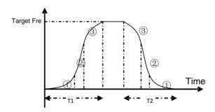
Fig 6-9 S curve acceleration /deceleration
