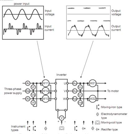
**Examples of Measuring Points and Instruments**
