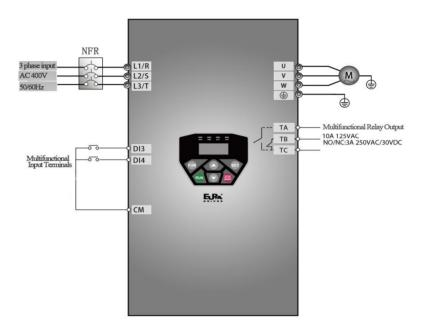
Figure 5-2 Wiring Diagram
