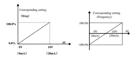
Fig 6-14correspondence of analog input to setting
