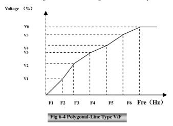
Note: during the process of speed track, polygonal-line V/F curve function is invalid. After speed track is finished, this function is valid.
